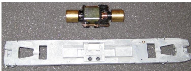
I next removed the brass clip, that holds the spring and brush which transfers the current to the commutator, on the bottom of the motor, being careful not to lose the spring and brush. I removed the two tabs that are punched out of the brass that make contact with the frame. This can be done by
