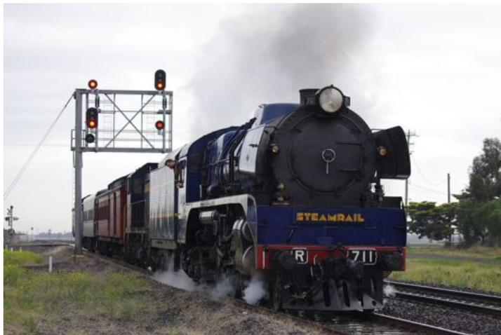
Engine #711 was equipped with 73 in drivers and measured 77 ft 3.5 in length. The weight on its drivers is 58 long tons (UK) or 65 short tons (US); this yields almost 22 short tons per driver axle. Total locomotive weight is 107 long tons or 120 short tons. Confused yet? That is why pictures are better than words.
