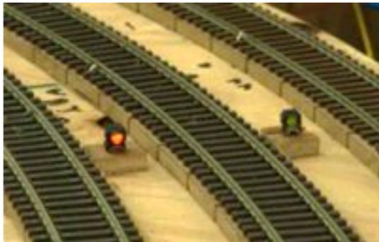
One set used a single lamp head with a bi-colored LED (Figure 1 to the left) and the other set had two lamp houses with a green and a red LED (figure 2 below left).
