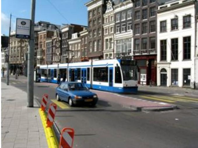
Power is picked up by pantograph (roof mounted and spring loaded) from overhead wires. Voltage is reported to be 600 or 750 V DC depending on the line.
