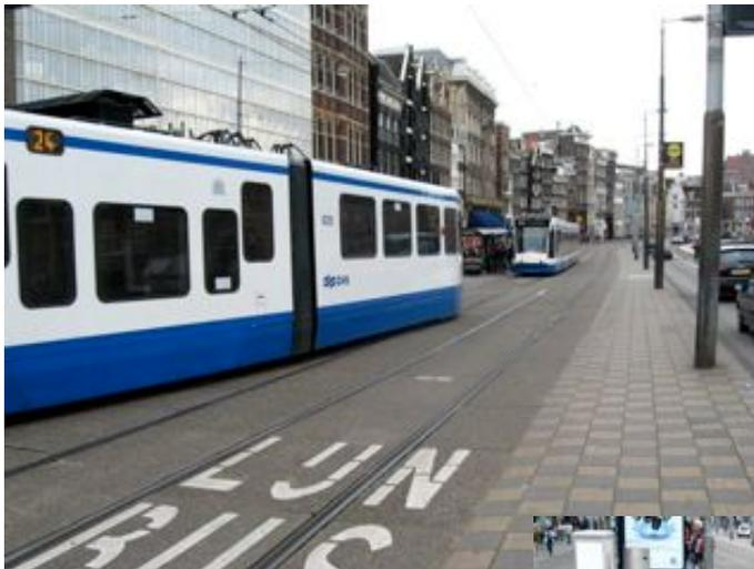
Note also the side skirting on the tram. Wheels are virtually out of sight. The trams are built with the external structure very close to the ground. This makes it very difficult to roll over a foot or have little children crawl under the tram cars at a stop.
