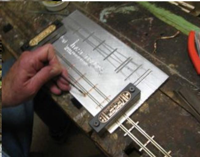
The bottom left photo shows how the gauntlet can be made to grow longer and longer. Hence a railroad builder can save bridge dollars and use a single bridge width and load arrangement for two tracks as long as his rail traffic is somewhat light and manageable.
