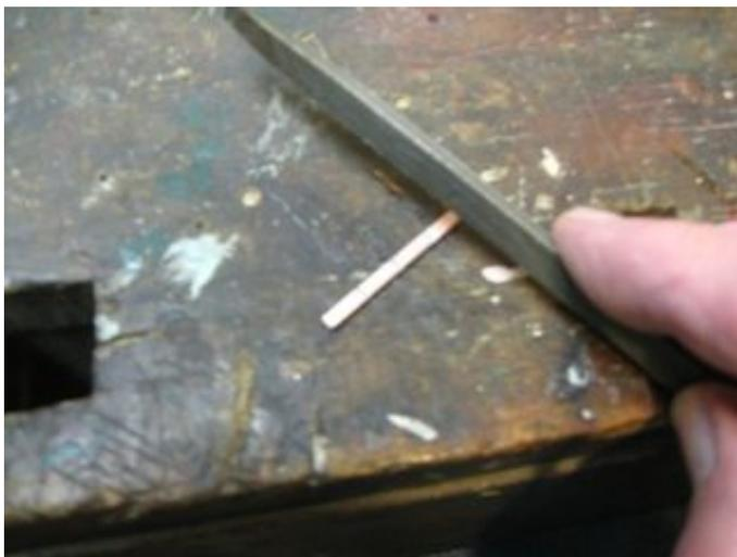
Making a gauntlet track is the simplest of the three types of trackage manufacturing I've tried. On the left I am using a triangular shape file and putting a shallow notch in a piece of copper clad fiberglass. The notch will prevent electrons to flow from one rail to another on the gauntlet. It's a simple chore and you'll find that one needs to cut three notches to provide electrical separation of the four gauntlet rails involved.
